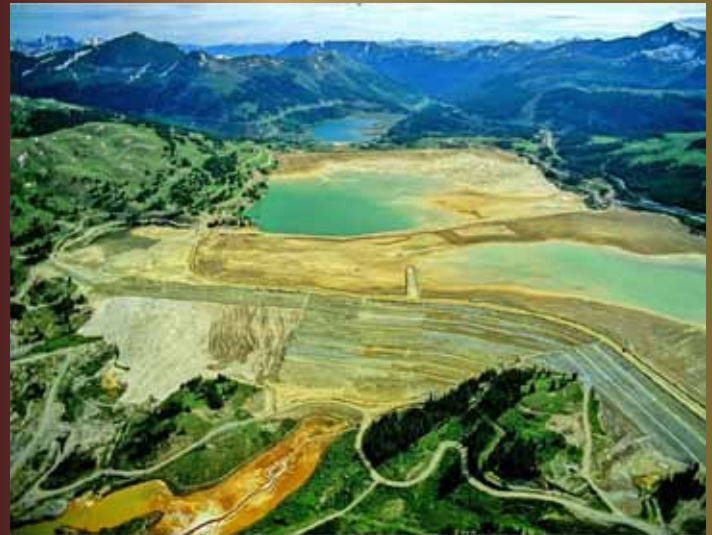
Figure 1. Climax Molybdenum Mine, Colorado. Operated as both open pit and underground facilities. Mine footprint is about 14,000 acres. Facilities have contaminated three rivers. About 3.2 billion gallons of contaminated water must be treated annually at a cost of about $4 million.
